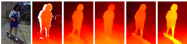
Figure 6: Ablations of depth quality. From left to right: input image, ground truth depth map, our full model ( full ), model without flow feature ( noflow ), model without upsampling supervision ( noupsu ) and model that do not drop out flow features ( nodrop ). See Section 4.5
