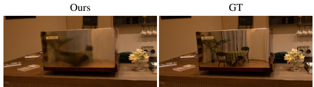
Figure 11. Our method cannot reconstruct mirror-like perfect reflections due to the limited capacity of the 3D Gaussian encoding.
